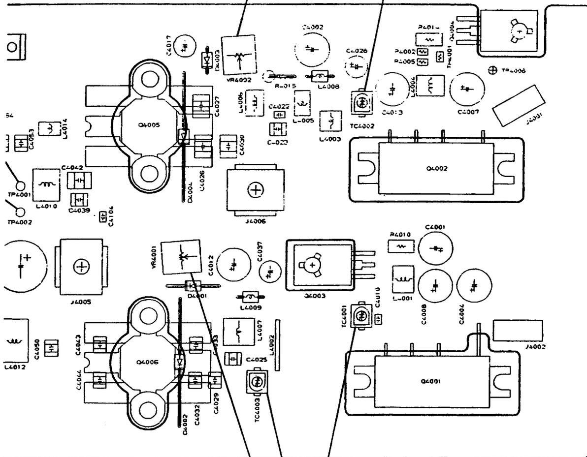
IF-PA Idling Current: Ammeter "+" lead ( $0.3 \pm 0.03A$ )
